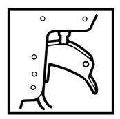
**SEQUENTIAL TRIP** Identified by **ORANGE TRIGGER**.
